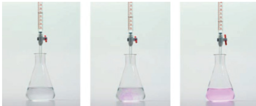
12.5-rasm. Tekshirilayotgan HCl ning miqdorini NaOHning ishchi eritmasi bilan titrlash. Indikator fenolftalien
